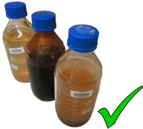
Figure 22 1 litre screw-top Pyrex/Schott glass bottles
