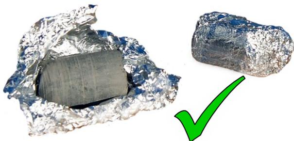
Figure 18 Side wall core in aluminium foil
