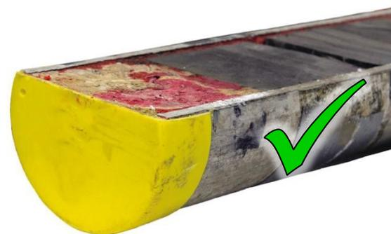
Figure 5 Tight fitting plastic end caps with cap cut to fit core barrel
