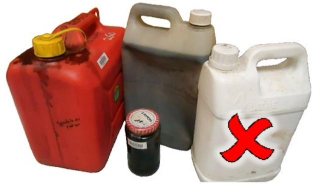
Figure 23 Example of unacceptable sample containers
