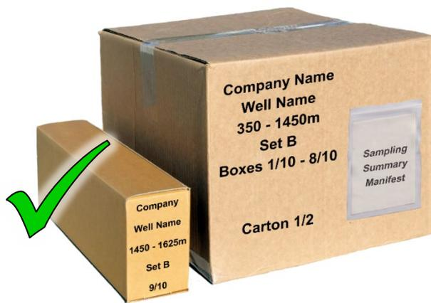
Figure 17 Correctly labelled smaller sample boxes and larger transport boxes
