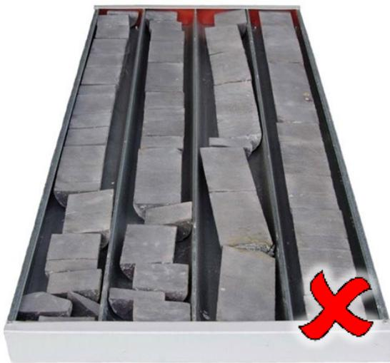
Figure 13 Undersize core for tray sections
