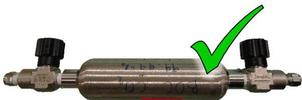
Figure 20 Gas cylinder: 150cc internal volume
