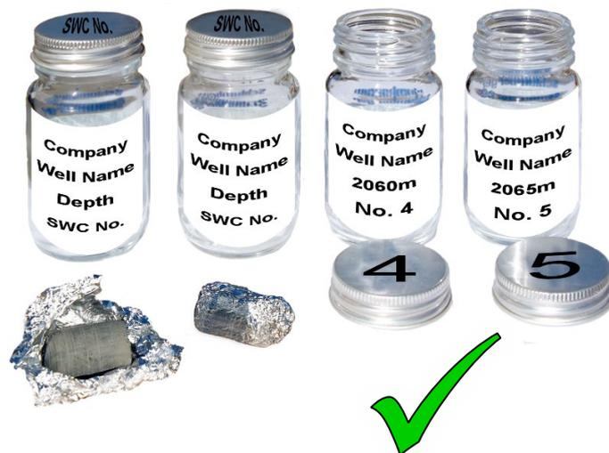
Figure 19 Correctly labelled side wall core jars with lids
