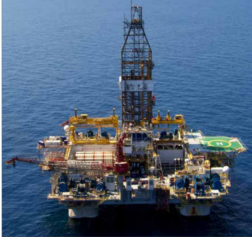
(left) Atwood Osprey Semisubmersible—image courtesy of Atwood Oceanics
